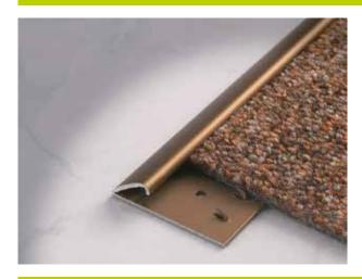
CARPETEC trim profiles compress to hold flexible flooring, such as natural fiber carpeting. By pressing the profiles, they close slightly to clamp the flooring, hiding and protecting edge imperfections.
